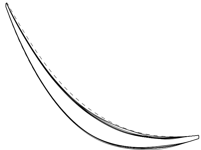
Fig. 7 Balanced designs from Table 4 showing variations in geometry, with base design shown dashed (shown distorted for clarity).
